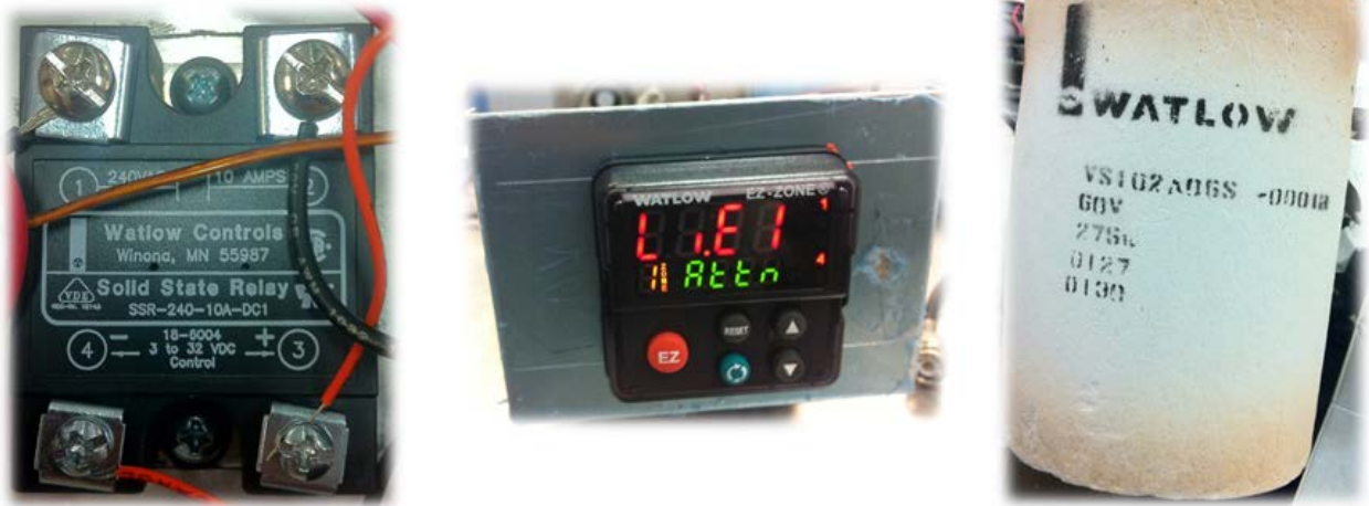
Figure 12: (left) Watlow solid state relay (middle) Watlow temperature control module (right) Watlow ceramic fiber heater
